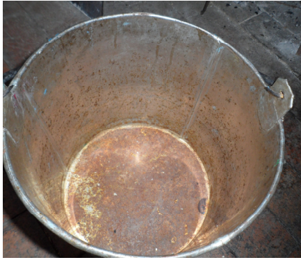
How a tin bucket looks when it's not properly dried after use.
